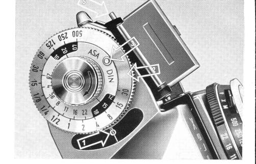
The shutter speeds to the left of  $^{1}/_{8}$  stand for fractions of seconds (thus 15 means  $^{1}/_{15}$  second), the figures to the right of  $^{1}/_{2}$  stand for full seconds.
