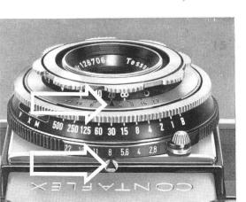
if you want to get a shot of children at play, set the aperture and shutter speed, and focus the lens at the most suitable distance. Now watch the view in the finder, and approach the subject until the two halves of the image in the rangefinder field coincide, or the picture is sharp on the ground glass ring. Then just check the view once more, and release.
