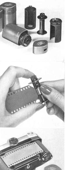
When working with two cassettes (Fig. 29) there is no need to rewind the film. It can also be unloaded after any number of exposures together with the take-up cassette in broad daylight. But advance the film by two frames before opening the camera. This two-cassette system is specially useful if you want to change over frequently from black-and-white film to colour and vice versa.
