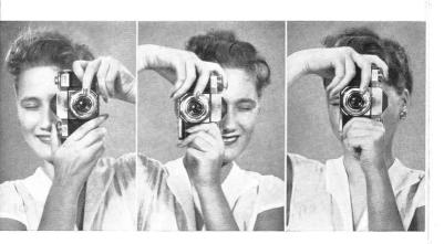
right hand the focusing mount (13). Use the left hand to support the CONTAFLEX II from below.
